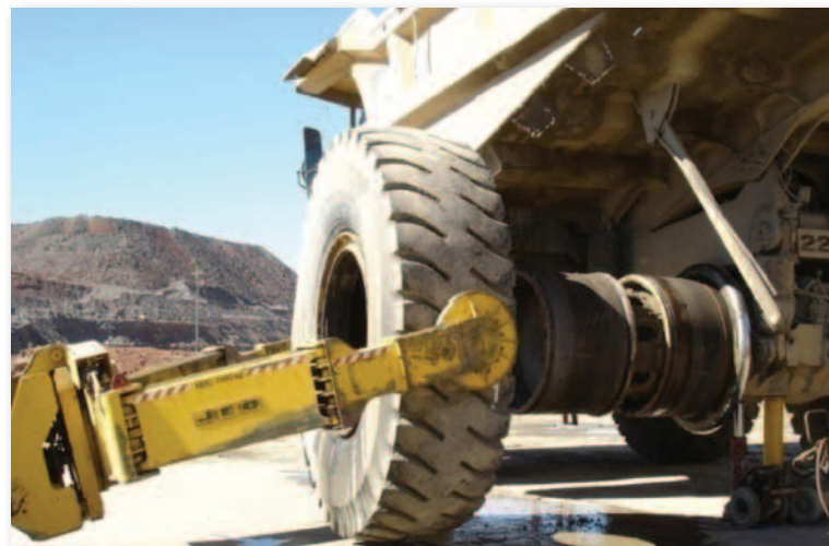
The smaller overall rim base diameter of the OVM, compared to the inside wheel, allows for the easy removal of the inside tyre and components over the OVM wheel base.
